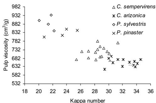
Fig. 7. Pulp viscosity vs kappa number.
