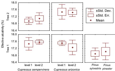
**Fig. 3.** Effective alkali consumption (as NaOH) for *Cupressus sempervirens*, *Cupressus arizonica*, *Pinus sylvestris* and *Pinus pinaster*.
