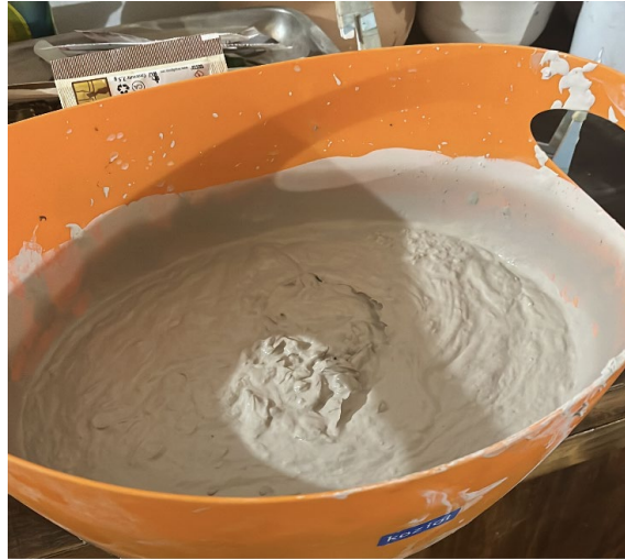
Fig. 2. A basin containing a paper-clay dough made with 2.5% cellulose paste and white clay.
