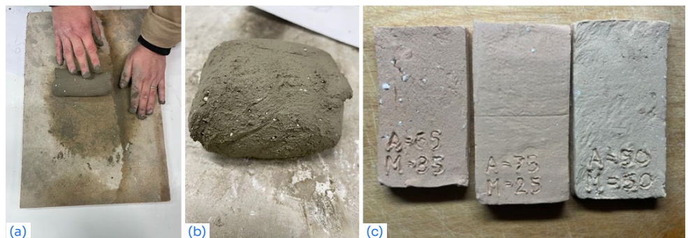
Fig. 1. (a, b) Clay mixture with calcium carbonate, in which the granules formed during the union of the two materials are visible; (c) The calcium carbonate granules still visible after firing three samples with different percentages of carbonate.
