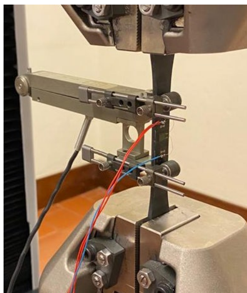
Figure 8. Clip-on extensometer and strain gauge glued to the specimen to be tested.
