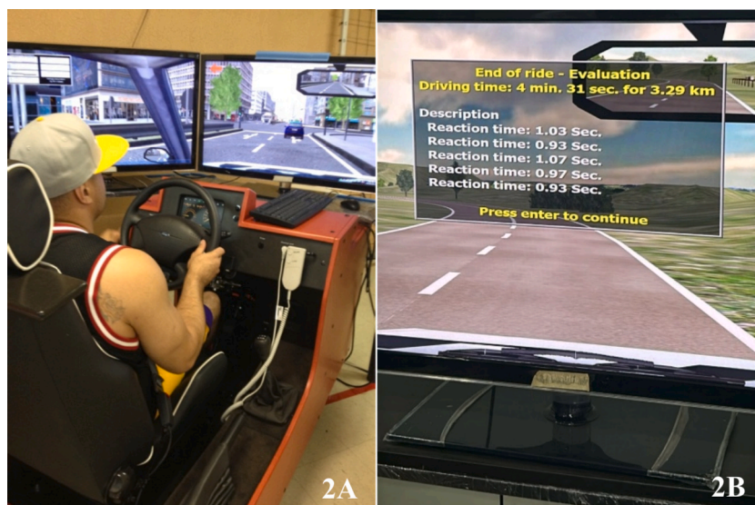
Fig. 2. – Car Simulator test routine. Fig. 2A - Driver engaged in the braking time task on the FOERST Car Simulator “Trainer” Type F12PT, a simulator with essential driving components in a virtual, single-lane environment without traffic. Fig. 2B - Scores from the braking time task and dual-task condition, comparing braking times with and without distraction during a structured conversation with the evaluator.
