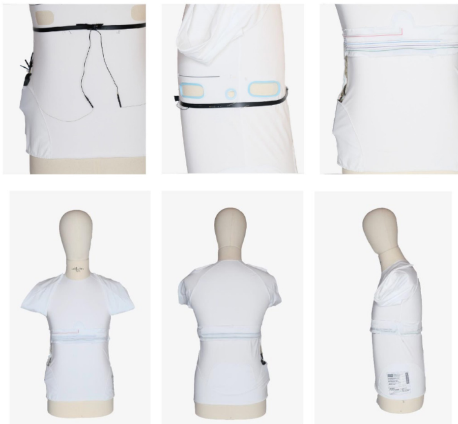
Fig.7 Smart&Safe Smart T-shirt, details. Focus on wearable add-on Smart T-Shirt. Focus on arrangement of conductive yarns by color and type of sensor connection; study of electronics components to operation and monitoring of vital parameters. Source: Smart&Safe Project, 2020
