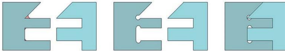
Figura 27 - Dog Bone Joint (Brasilia Fab Lab,2017a).
