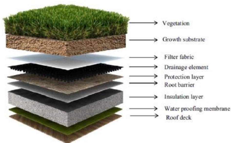
Figure 5 - Schematics of different layers (Besir & Cuce, 2018).
