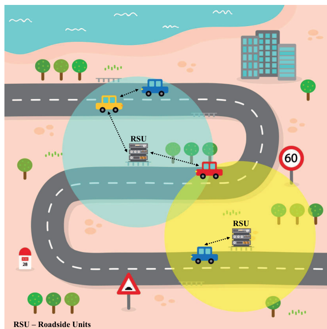
Figure 1. Example of a vehicular network scenario, considering both types of communication between nodes (V2V and V2I), where mobility management functions are needed to enable communication between different groups of mobile nodes.
