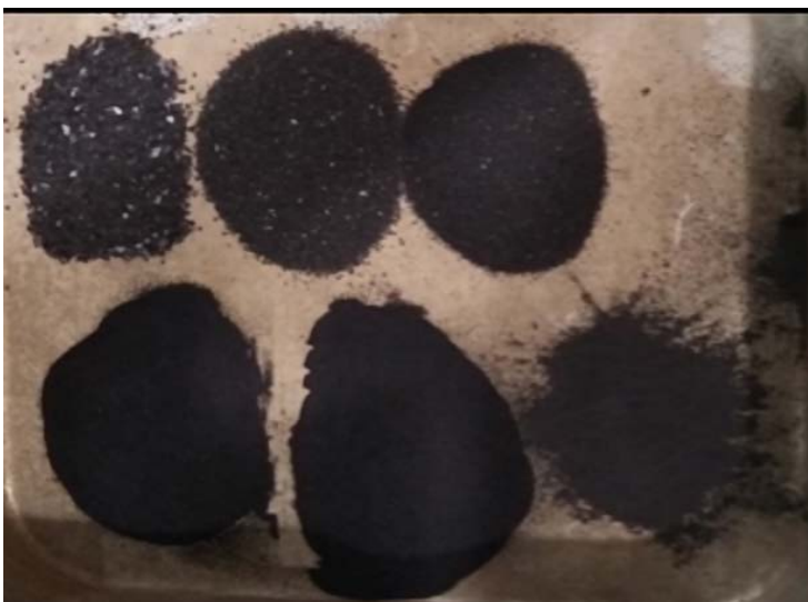
Figure 4 Dregs - particles after sieving separation
