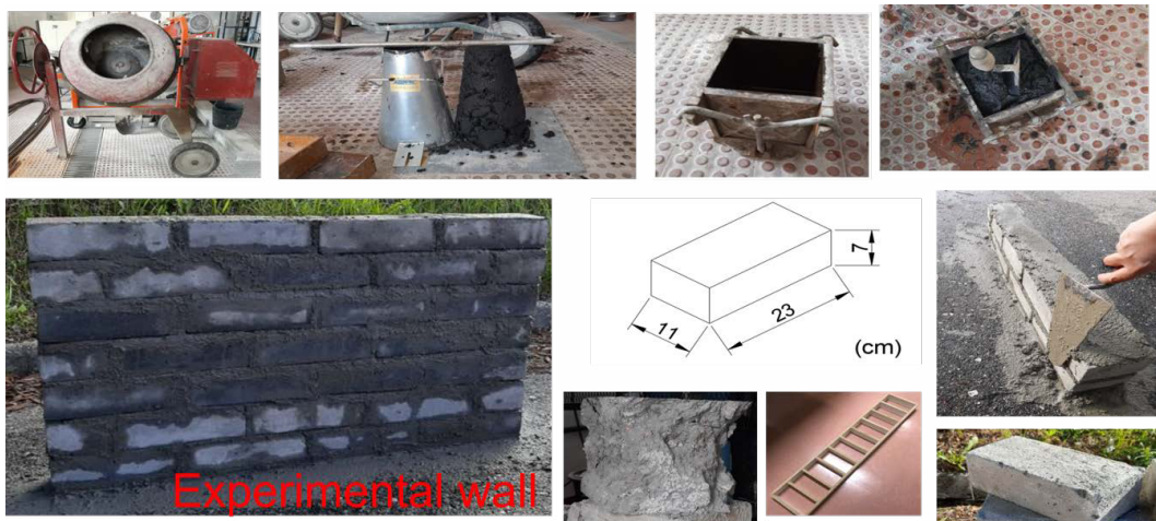
Figure 5 Stages of the laboratory methodology and experimental prototype wall
