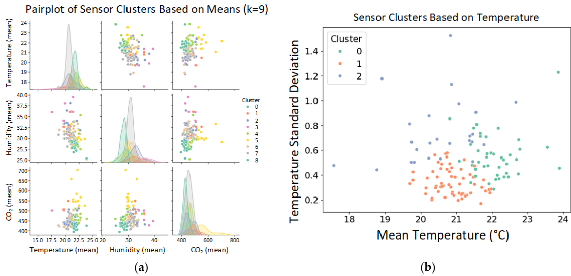
Figure 8. Pairplot of sensor clusters ( k = 9 ) on the left side (a). Result of all temperature sensor data clusterization on the right side (b).
