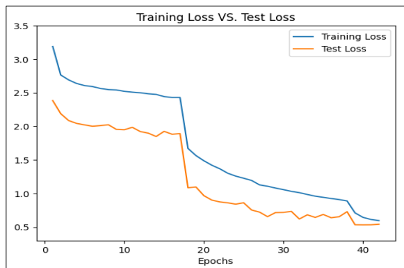
Fig. 16: Results of the ResNet-50 training process for the training loss and test loss metrics
