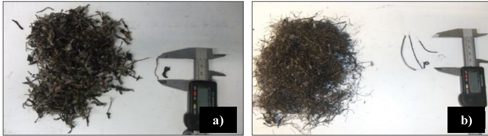
Figure 1: Recycled fibers from tires. a) Textiles fibers. b) Steel fibers
