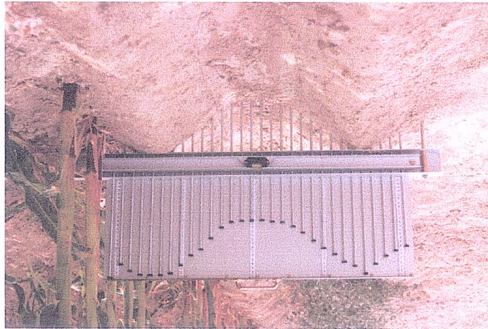
Fig.6 - Profilometer for register of the furrow cross-section.
