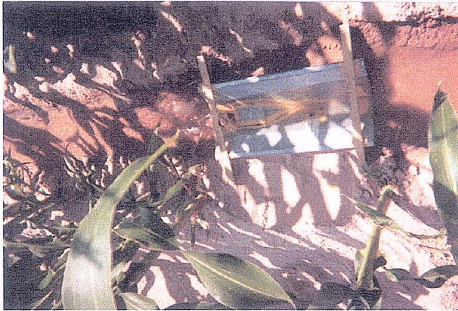
Fig.2 - Portable trapezoidal flume (Replogle and Bos, 1982).
