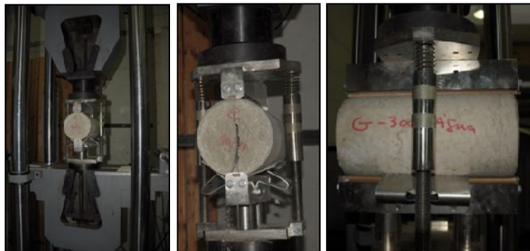
Figure 6: Test set-up – residual splitting tensile strength tests
