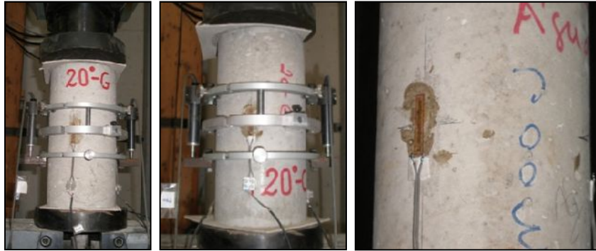
Figure 8: Test set-up – residual modulus of elasticity tests
