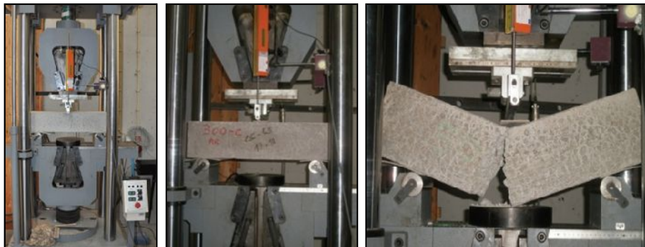
Figure 7: Test set-up – residual flexural strength tests
