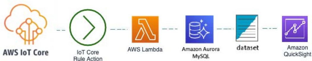
Figure 5 AWS IoT Analytics to prepare data for QuickSight.
